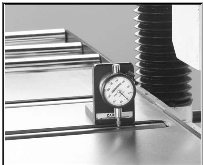
Figure 35. Measuring table roller height with Rotacator® in downward position.
