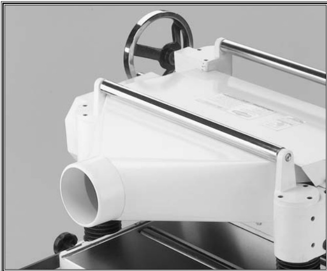
Figure 5. Dust hood attached to planer.
