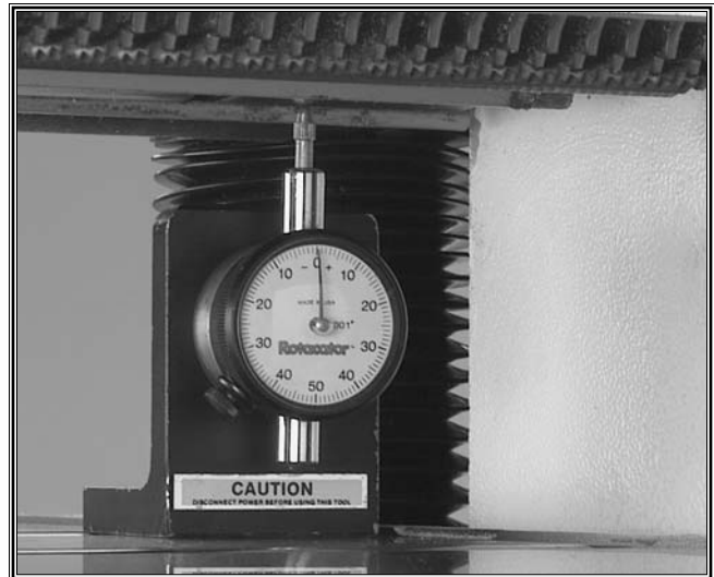
Figure 34. Measuring table-to-cutterhead with Rotacator® in upward position.
