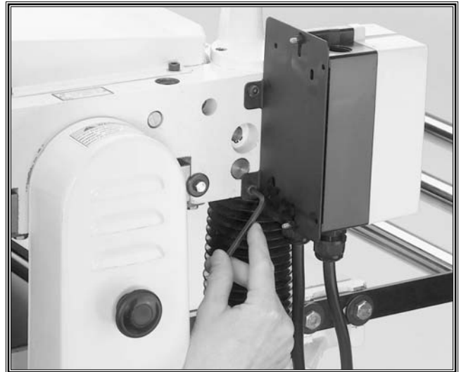
Figure 6. Attaching switch to the planer.
