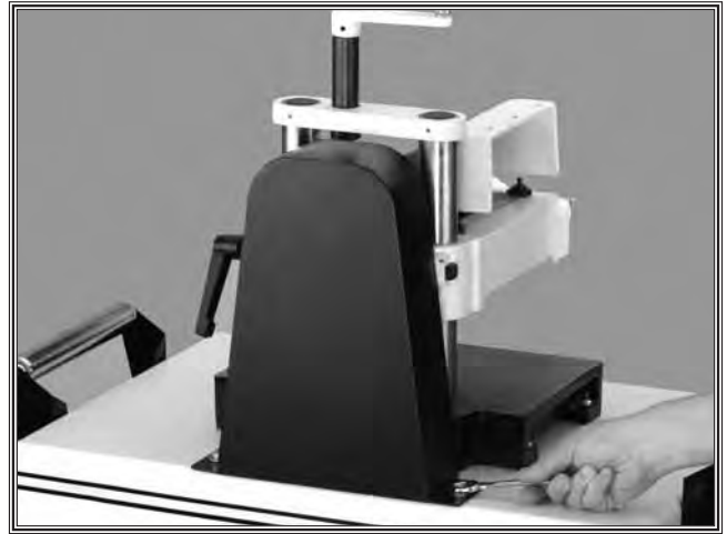
Figure 17. Installing the belt guard.
