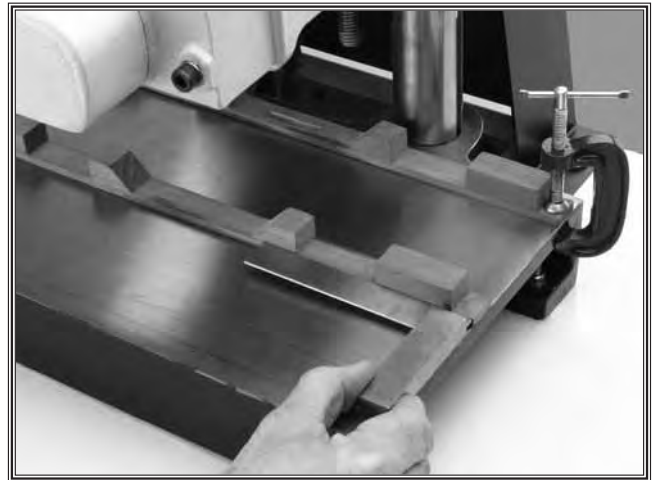
Figure 32. Fences aligned to the work table.
