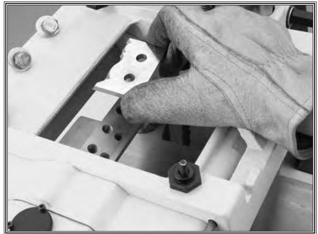
Figure 30. Moulder knife installation.
