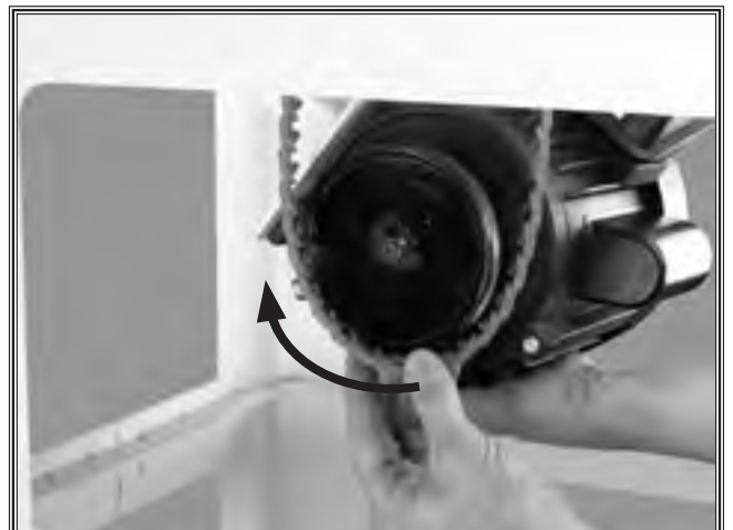
Figure 13. Installing the drive belt (Belt cover removed for clarity).
