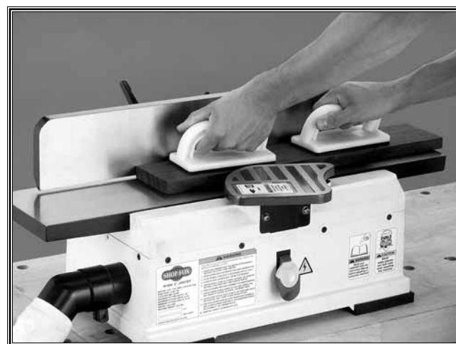
Figure 33. This is an example of a surface planing operation.
