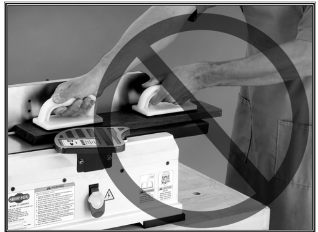
Figure 3. Never stand directly behind the workpiece!
