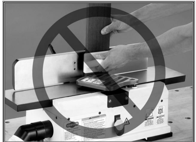
Figure 5. Never joint end grain!
