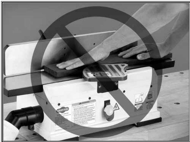
Figure 2. Never surface plane without push blocks!
