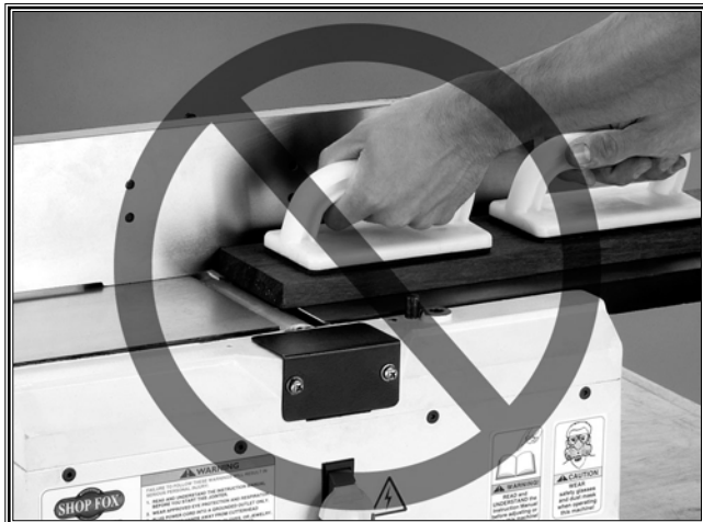
Figure 4. Never plane/edge-joint with the guard removed!
