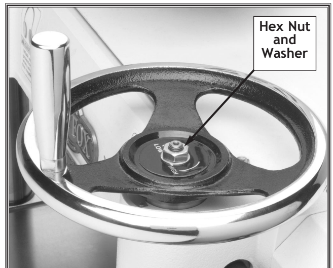
Figure 5. Installed handwheel and handle.
