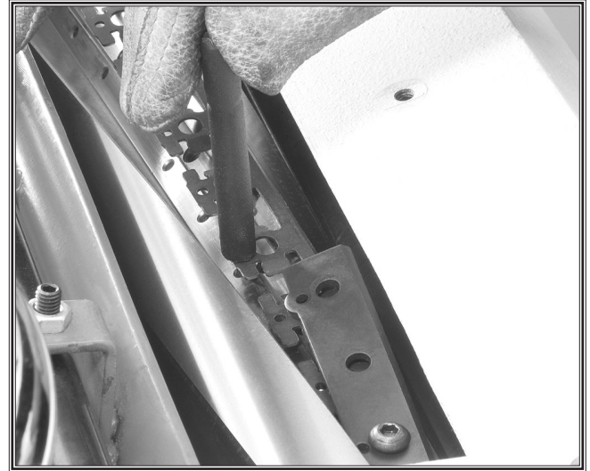
Figure 24. Twisting knife and aligning gib.
