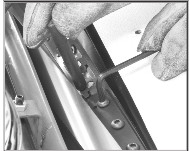
Figure 25. Keeping tangs in alignment groove.
