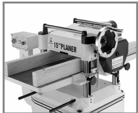
Figure 39. Gauge boards installed.
