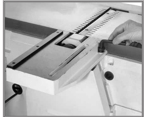
Figure 12. Installing fence bracket.
