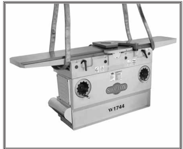
Figure 10. Model W1744 supported evenly by two lifting straps.
