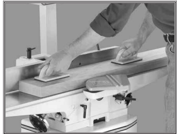
Figure 30. Typical surface planing operation.
