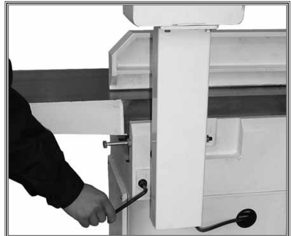
Figure 16. Mounting pedestal in upright position.
