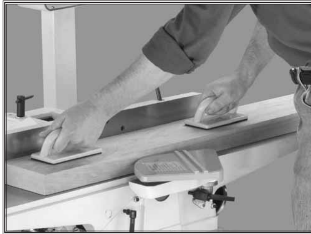
Figure 2. Correct operator and workpiece position, guard is in place, and push blocks are being used.
