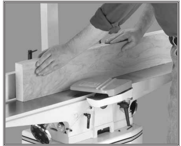
Figure 32. Typical edge jointing operation.
