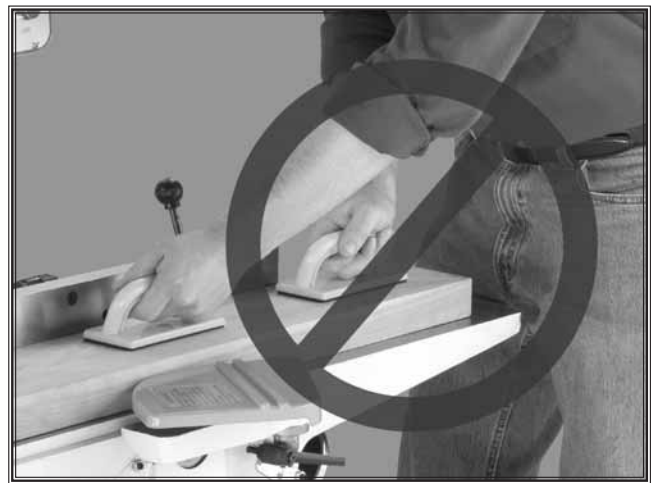
Figure 5. Never stand directly behind the workpiece!
