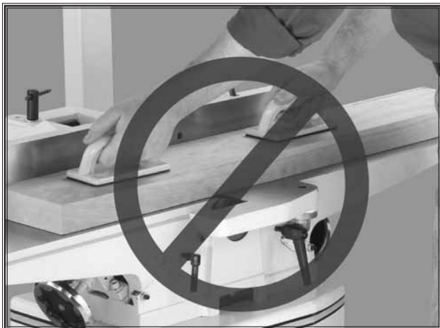
Figure 4. Never plane/edge-joint with the guard removed!
