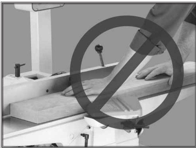
Figure 3. Never surface plane without push blocks!
