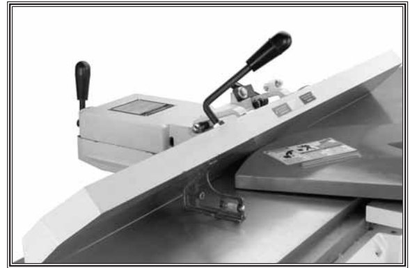
Figure 53. Fence adjusted 45° inward.
