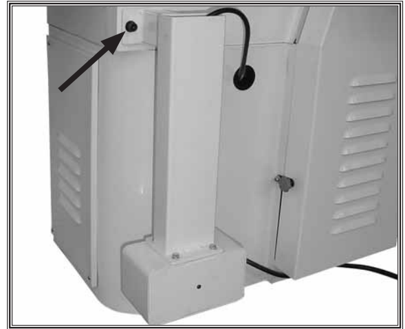
Figure 15. Location to remove pedestal mounting hardware (one side shown).
