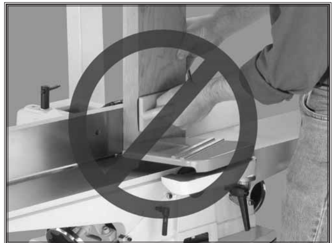
Figure 6. Never joint end grain!
