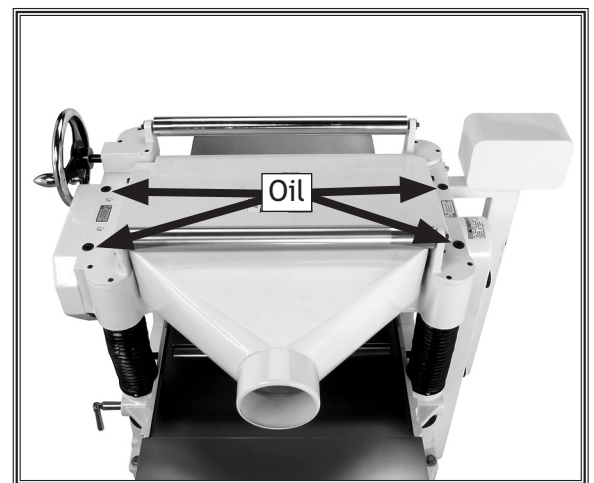
Figure 16. Feed roller lubrication locations.
