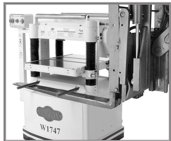
Figure 3. Example of planer being lifted using forklift.
