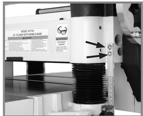
Figure 36. Depth scale adjustment screws.
