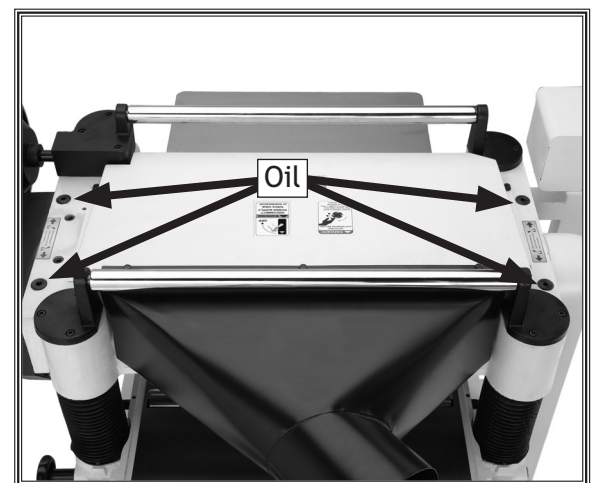
Figure 19. Feed roller lubrication locations.
