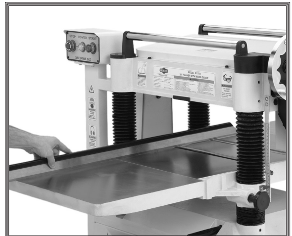
Figure 6. Example of leveling extension wings and table.
