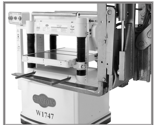
Figure 4. Example of planer being lifted using forklift.
