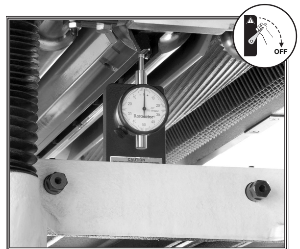
Figure 29. Finding BDC with the Rotacator.
