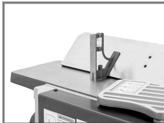
Figure 44. Checking the outward 45° stop.
