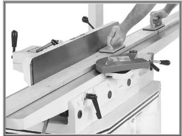
Figure 34. Typical surface planing operation.
