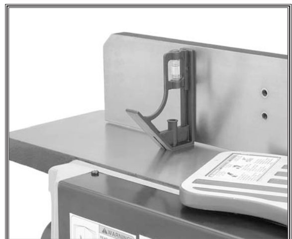
Figure 41. Checking the 90° stop.
