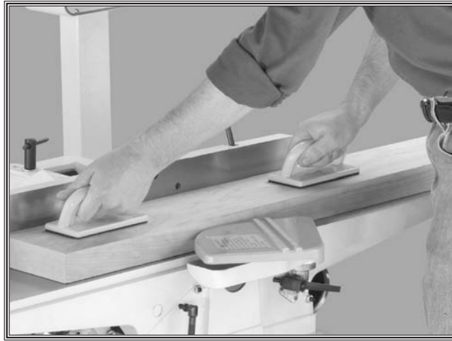
Figure 3. Correct operator and workpiece position, guard is in place, and push blocks are being used.
