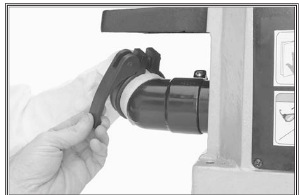
Figure 24. Attaching the dust collection bag.
