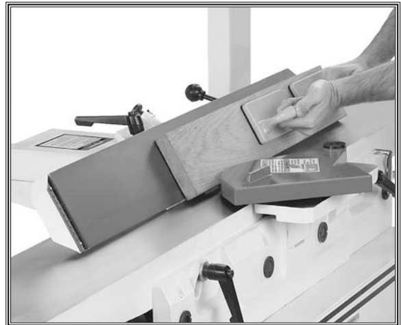
Figure 38. Typical bevel cutting operation.
