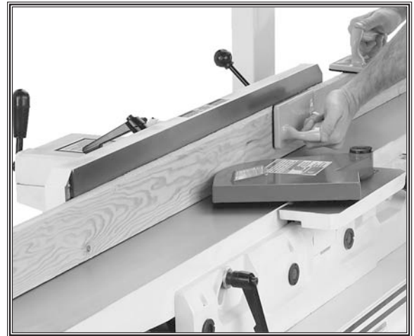
Figure 36. Typical edge jointing operation.
