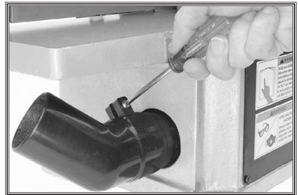
Figure 23. Installing the dust chute.
