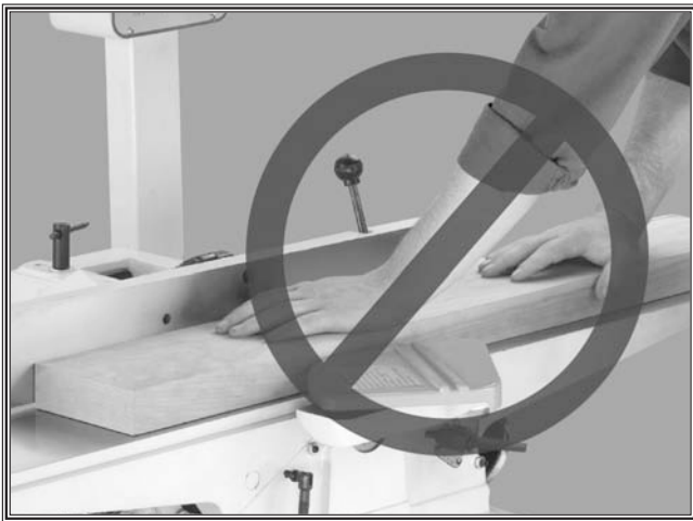
Figure 4. Never surface plane without push blocks!
