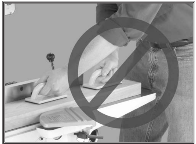
Figure 6. Never stand directly behind the workpiece!
