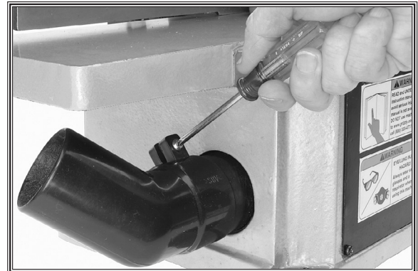
Figure 16. Installing the dust port.
