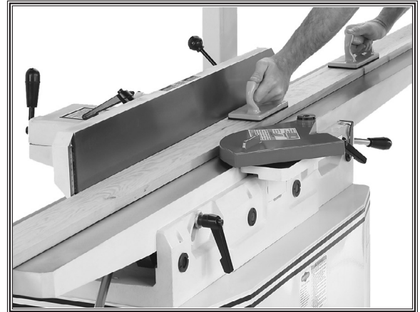
Figure 30. Typical surface planing operation.
