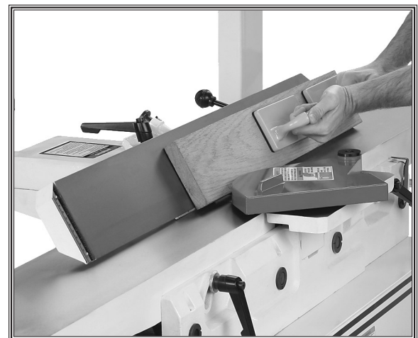
Figure 35. Typical bevel cutting operation.
