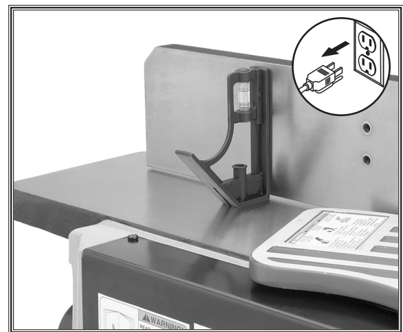
Figure 44. Checking the 90° stop.
