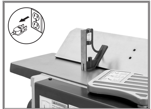
Figure 47. Checking the outward 45° stop.
