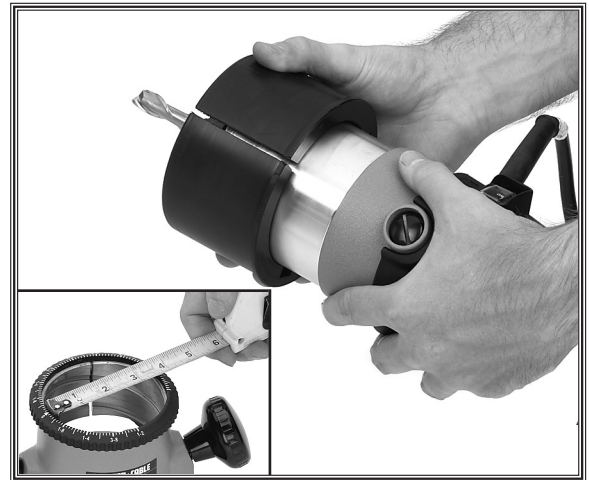
Figure 9. Fitting correct size adapter onto router motor.
