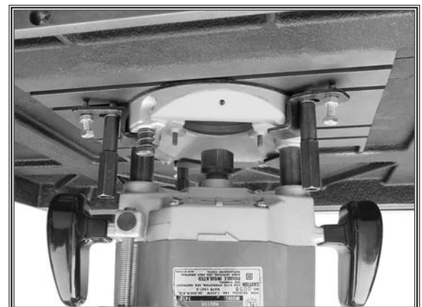
Figure 18. Router properly installed.
