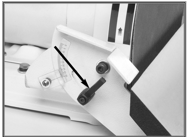
Figure 8. Installed tilting knobs.
