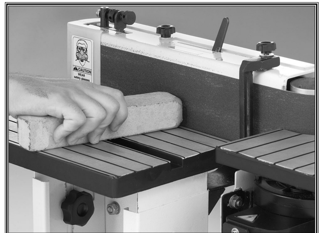
Figure 27. Cleaning the sanding belt with PRO STICK®.
