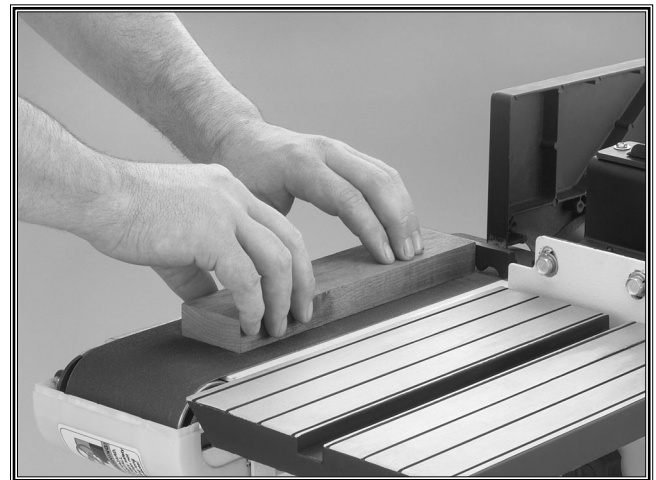
Figure 21. Flat sanding operation.
