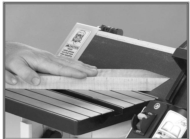
Figure 23. Contour sanding operation.
