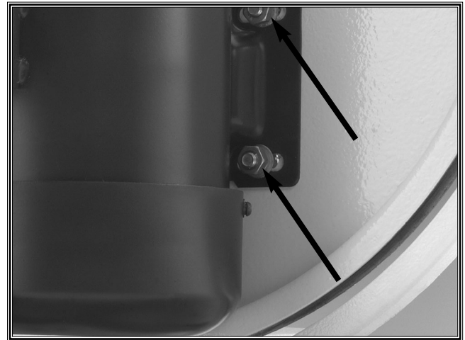
Figure 12. Motor mounting bolts (only 2 shown).
