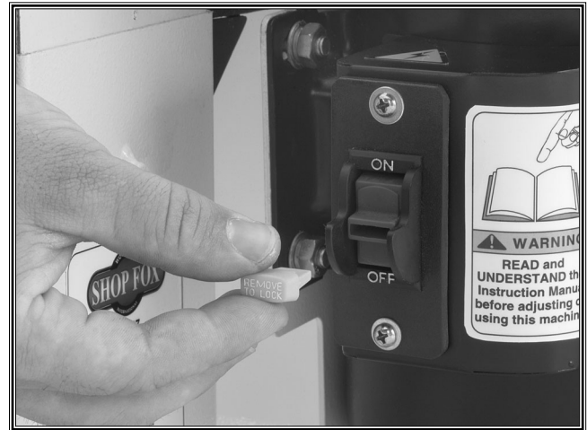
Figure 14. Safety lockout key removed.
