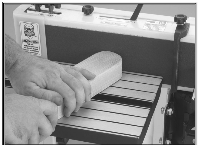
Figure 17. End sanding operation.
