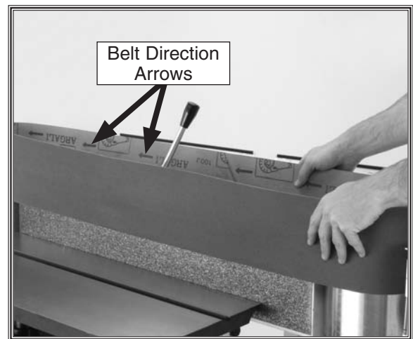
Figure 12. Placing the sanding belt onto the sanding drums.
