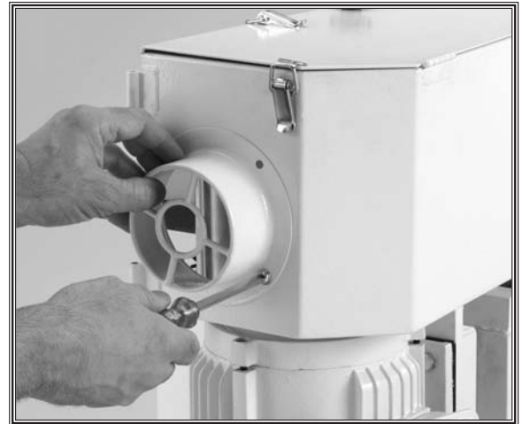
Figure 14. Dust port installation.
