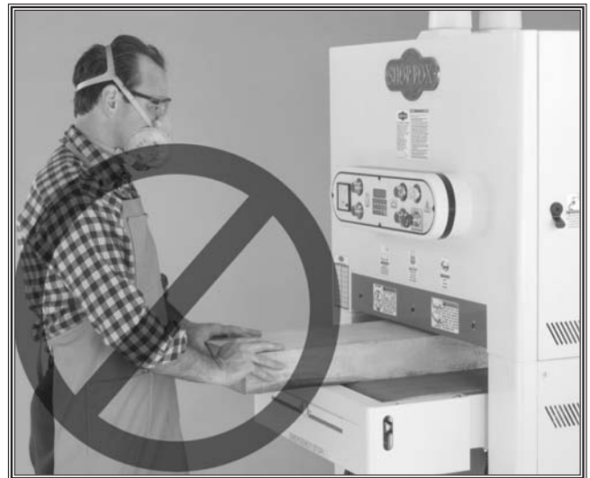
Figure 4. DO NOT stand behind workpiece!
