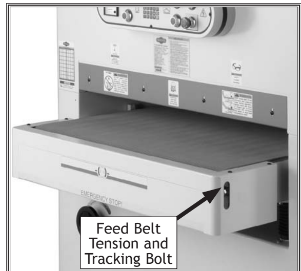
Figure 47. Feed belt tension bolt.
