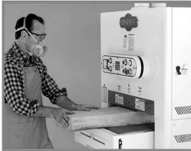
Figure 1. Correct body and hand positioning.
