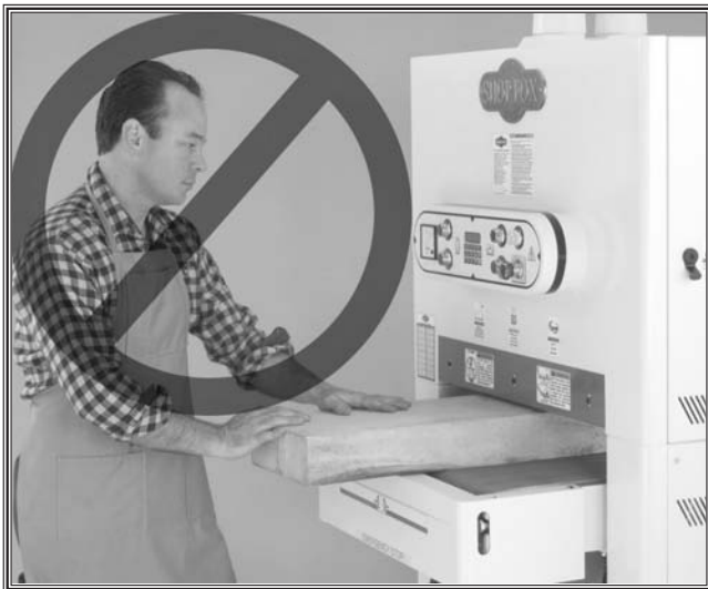
Figure 2. DO NOT operate without safety glasses/respirator!
