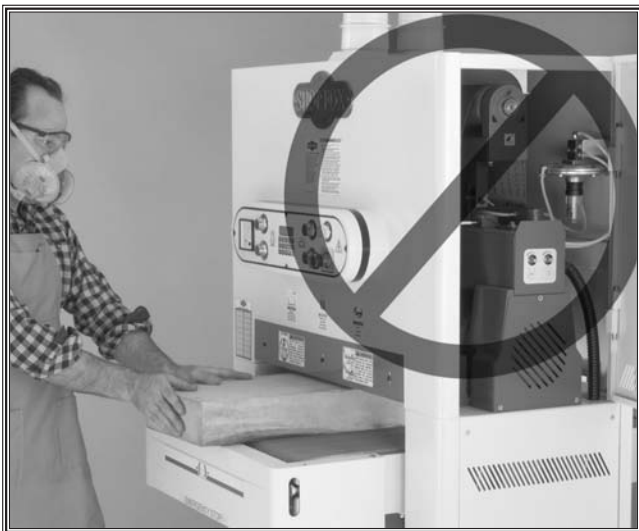
Figure 3. DO NOT operate with side door open!
