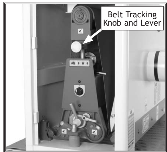
Figure 26. Belt tracking adjustment.
