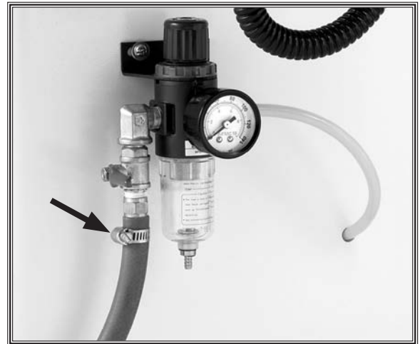
Figure 10. Air hose attached to regulator.
