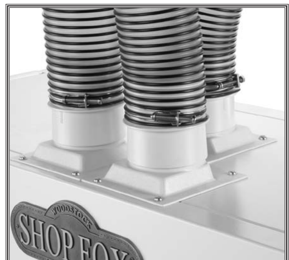
Figure 15. Dust collection hose attached to dust port.
