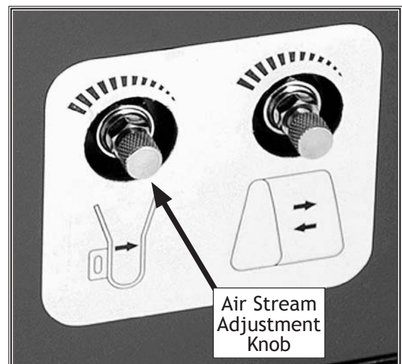
Figure 24. Air Stream adjustment knob.
