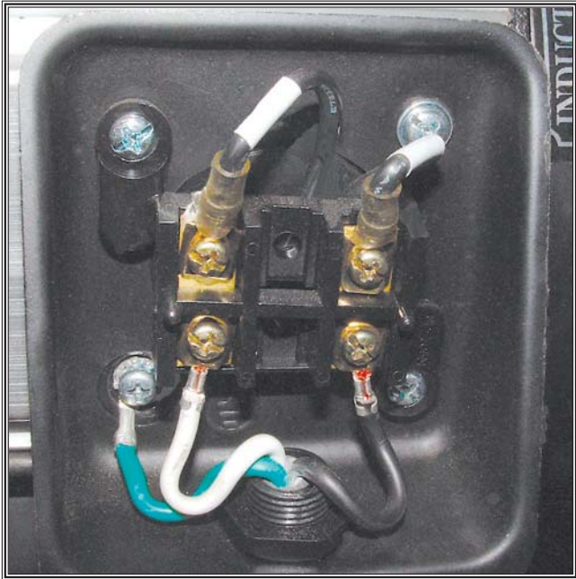
Figure 42. Sanding motor wiring.
