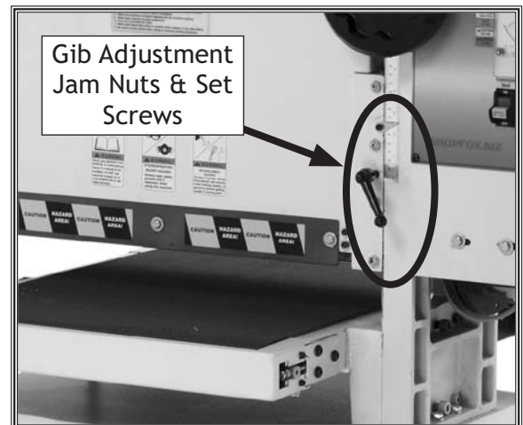
Figure 29. Gib adjustment jam nuts and set screws.
