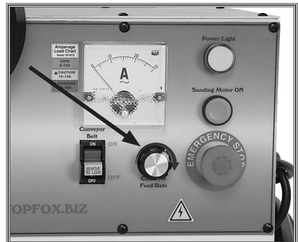
Figure 20. Conveyor feed rate dial.
