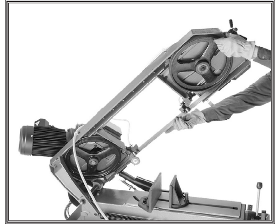
Figure 33. Typical blade installation.
