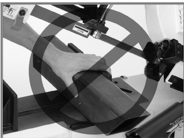
Figure 5. Never hold the workpiece by hand.
