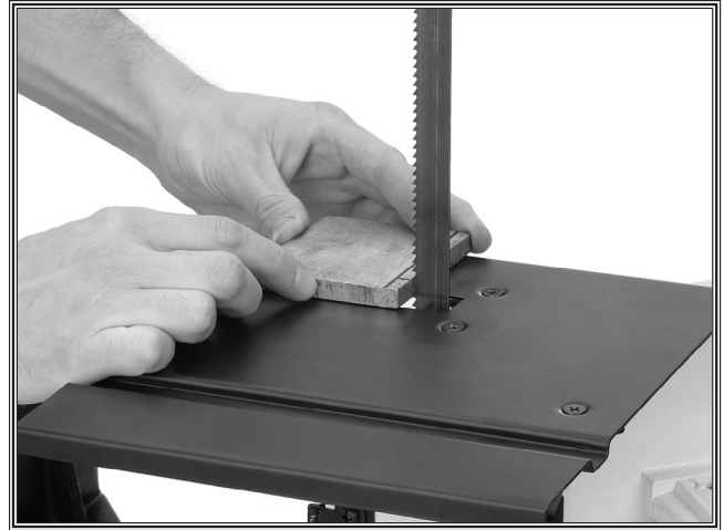
Figure 6. Always use the table for freehand cutting and keep fingers clear of blade.
