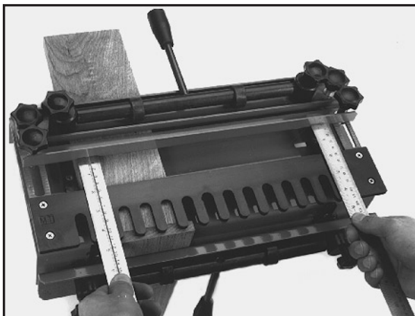
Figure 10 shows checking the alignment of the fence.
