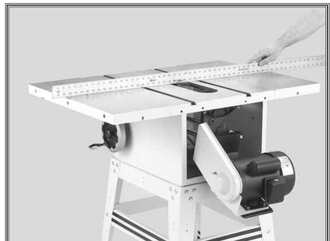
Figure 27. Checking both wings after assembly.
