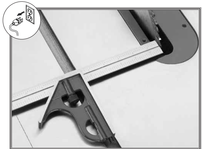
Figure 42. Checking blade/miter slot parallel.
