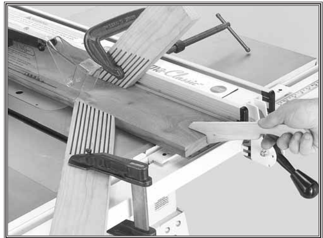
Figure 66. Use a push stick when ripping narrow pieces.
