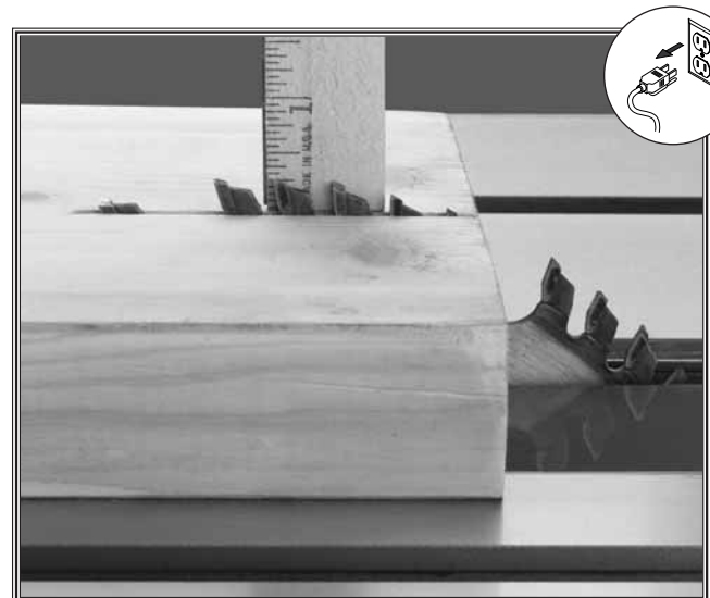
Figure 64 Blade protruding \frac{1}{4} " from workpiece.
