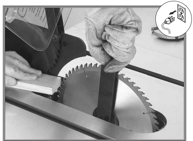
Figure 41. Tightening blade (from behind the machine).
