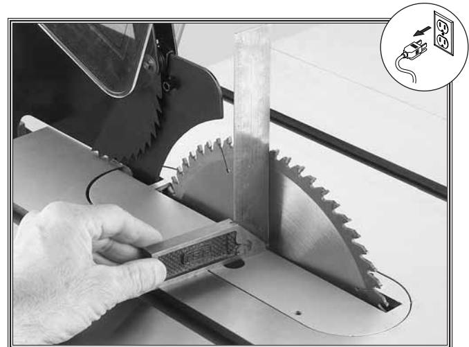
Figure 52. Setting blade to 90°.
