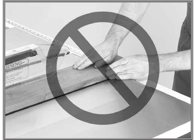
Figure 3. NEVER not freehand cut on a table saw.
