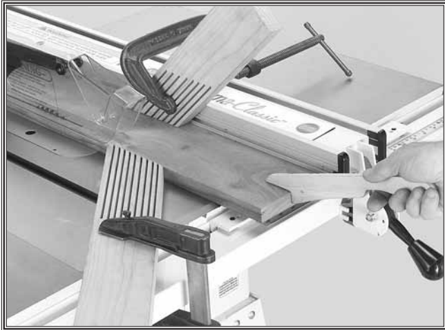
Figure 2. ALWAYS support your workpiece during a cut.
