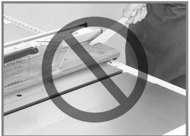
Figure 7. NEVER stand directly behind blade when making a cut.
