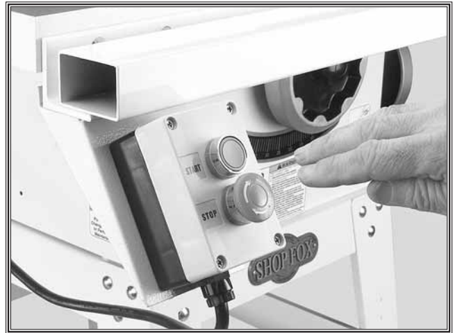
Figure 57. Hand poised over ON/OFF switch.
