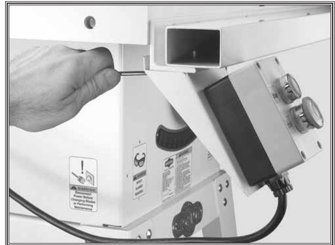
Figure 37. Installing ON/OFF switch.
