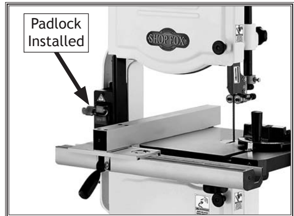
Figure 34. Padlock installed in the switch.
