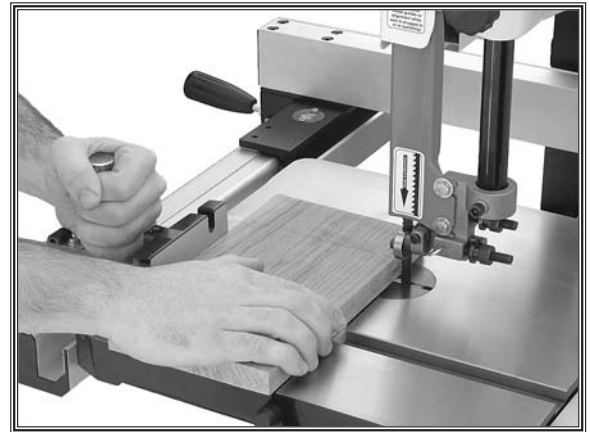
Figure 43. Making a 90° crosscut.
