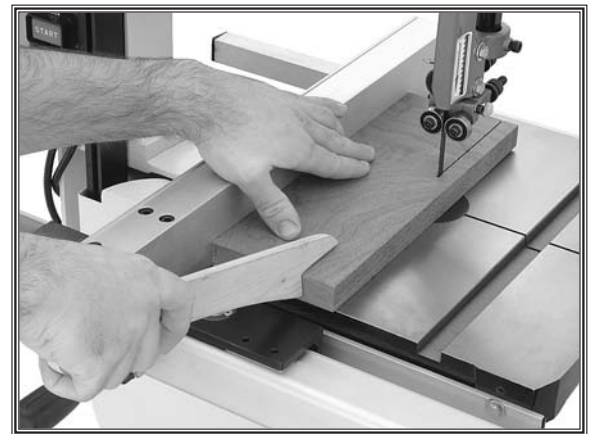
Figure 42. Example of ripping.
