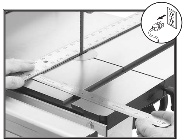
Figure 21. Taking measurements for aligning the table with the blade.
