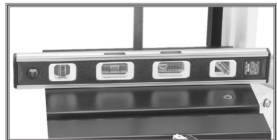
Figure 25. Adjusting table with a level.
