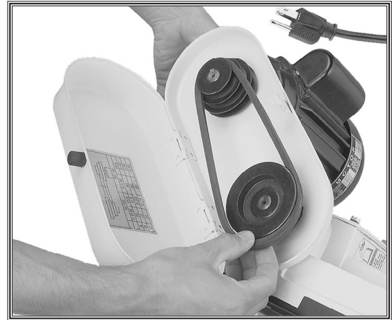
Figure 52. Installing the V-belt.
