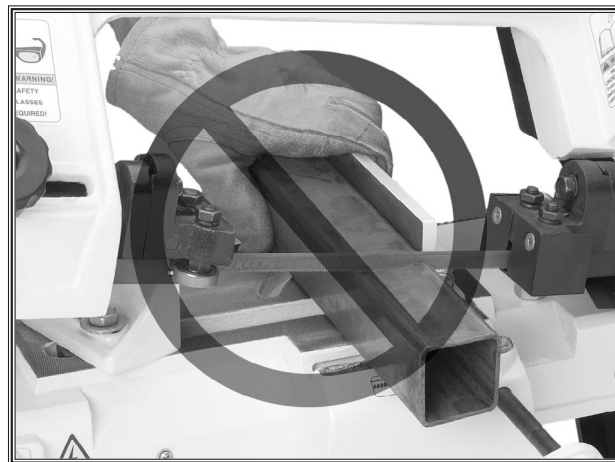
Figure 4. Never cut without using the vise in the horizontal position.
