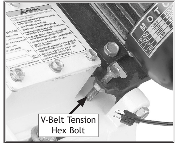
Figure 51. V-belt tension hex bolt.
