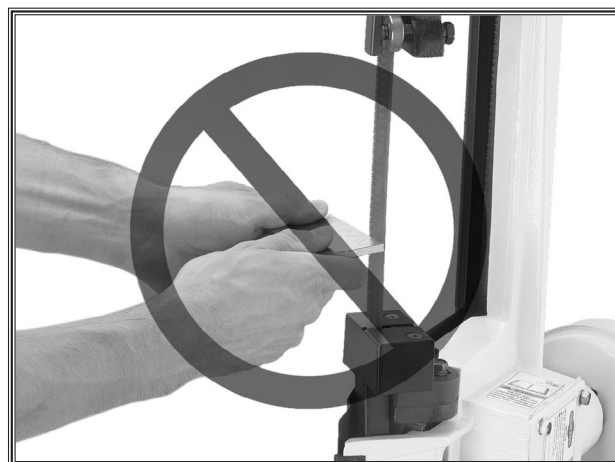
Figure 5. Never cut material "free-hand" in the vertical position.
