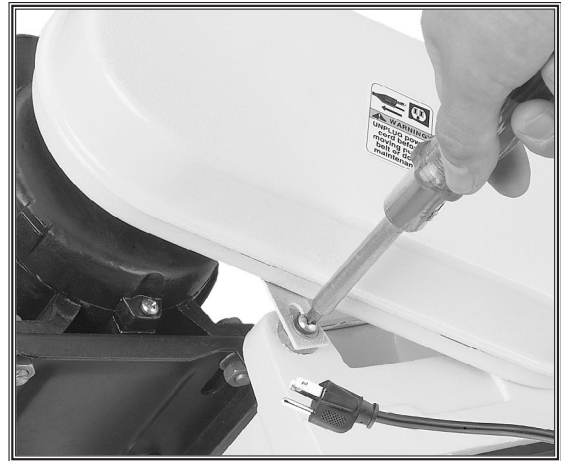
Figure 13. Installing the pulley cover.
