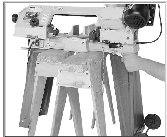
Figure 11. Attaching leg assemblies.
