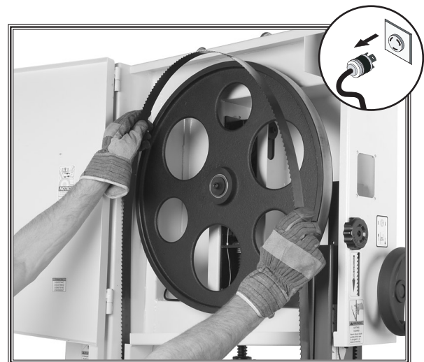
Figure 62. Typical example of placing blade on the wheels.
