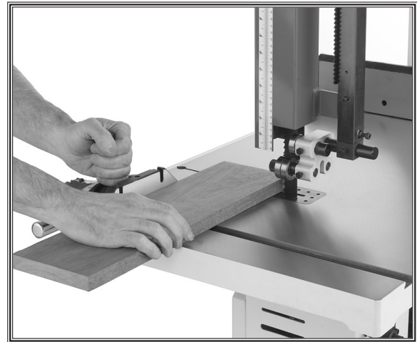
Figure 56. Typical crosscutting operation.
