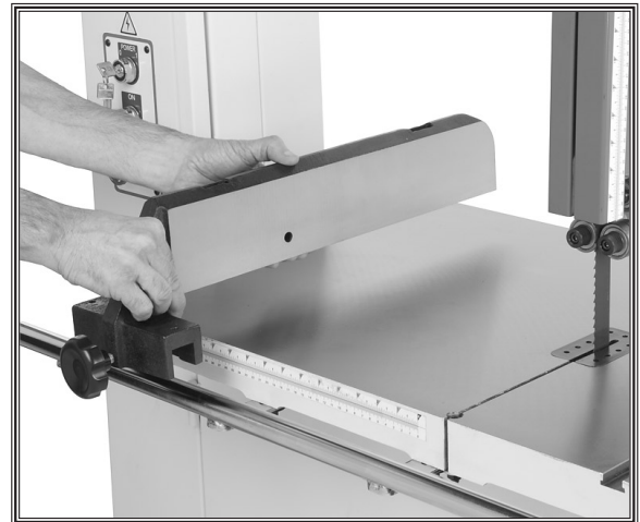
Figure 15. Installing fence onto rail.
