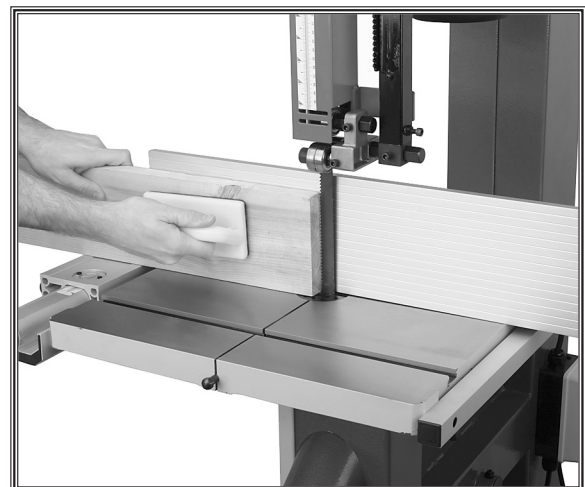
Figure 57. Example of resawing lumber.
