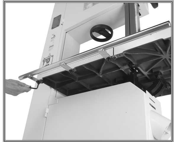
Figure 14. Tightening guard rail cap screws.
