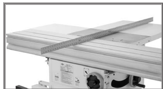
Figure 16. Extension wings mounted and even with cast iron table.
