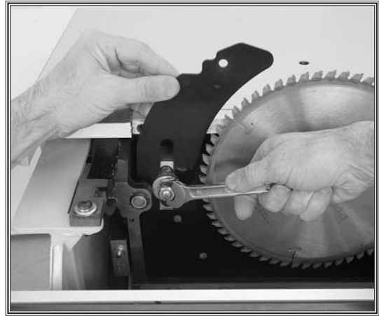
Figure 36. Installing riving knife.
