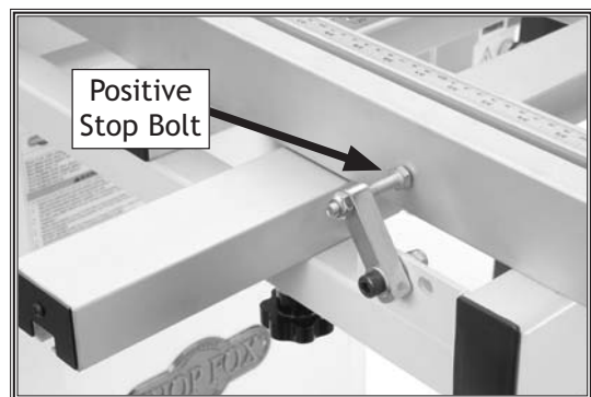
Figure 26. Positive stop bolt against the crosscut fence.
