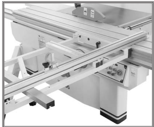
Figure 78. Example of miter cutting operation (0° to 90°).
