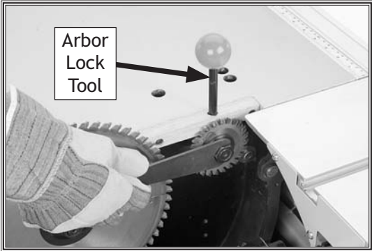
Figure 35. Installing scoring blade.
