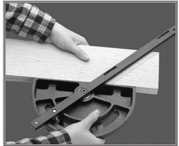
Figure 53. Example of marking miter line.
