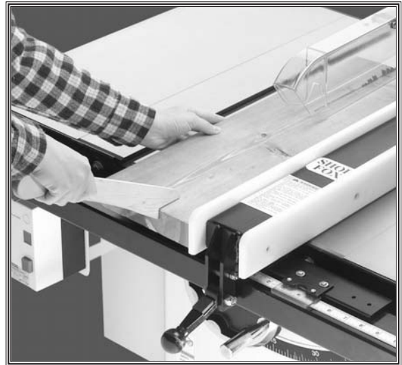
Figure 51. Typical ripping operation.
