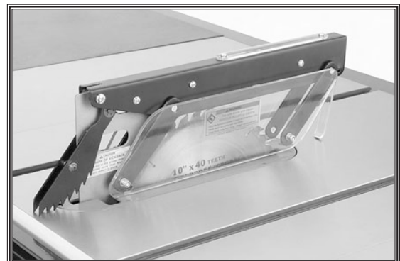
Figure 31. Blade guard installed.
