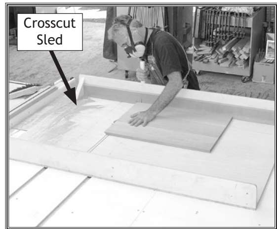
Figure 89. Example of crosscut sled.
