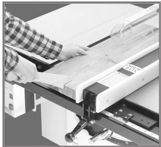
Figure 51. Typical ripping operation.
