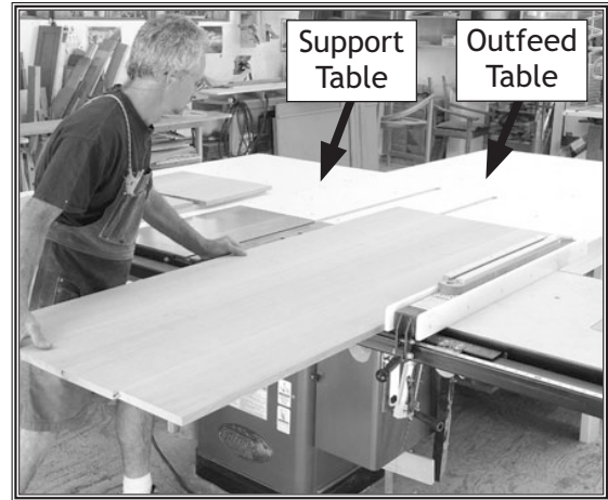
Figure 88. Example of outfeed & support tables.
