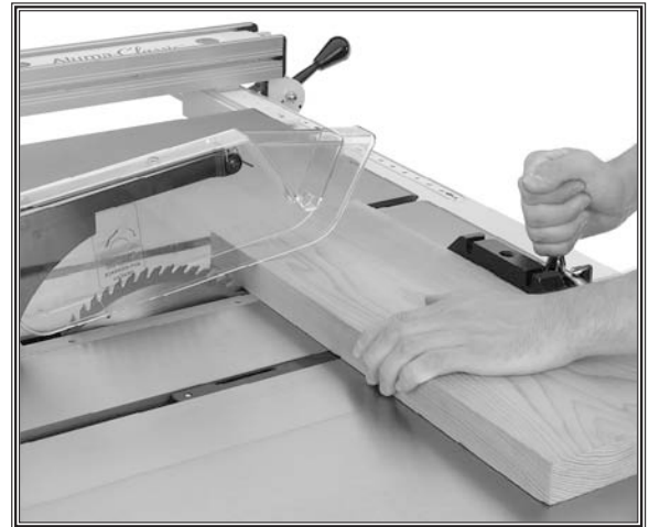
Figure 46. Example photo of a crosscutting operation.
