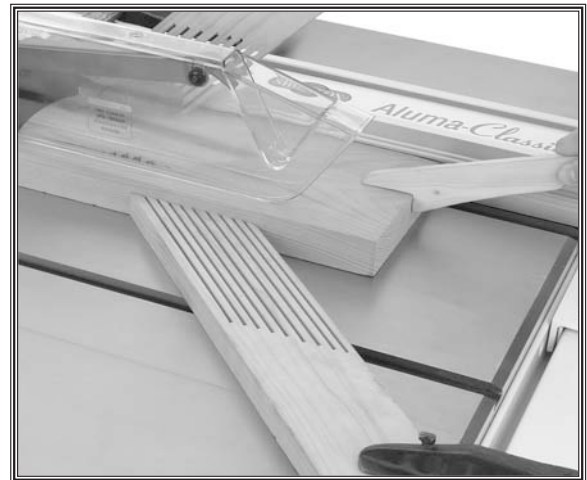
Figure 45. Example photo of a ripping operation.
