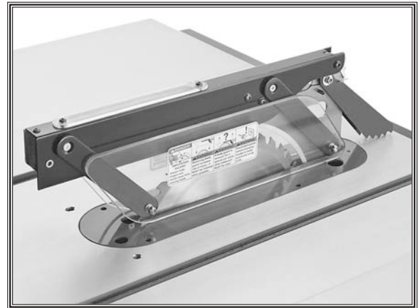
Figure 39. Blade guard and spreader properly installed.
