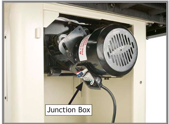
Figure 111. Motor junction box location.
