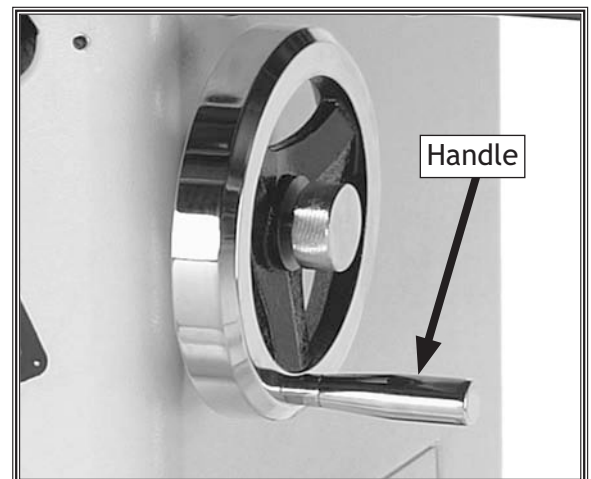
Figure 13. Handwheel handle installed.
