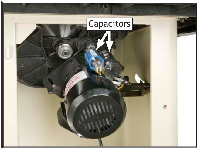
Figure 110. Motor capacitor location.
