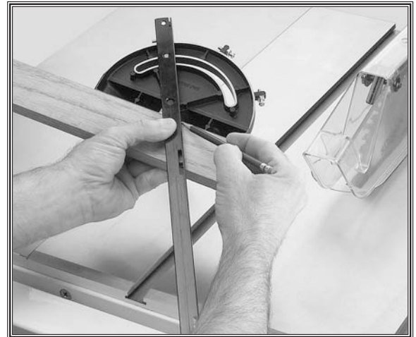
Figure 47. Example photo of making a miter mark.
