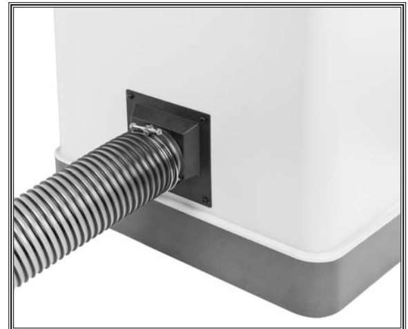
Figure 24. Dust hose secured to the table saw.
