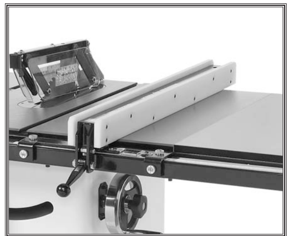
Figure 21. Fence assembly installed.
