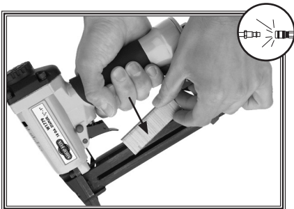
Figure 4. Loading staples into magazine. -8-
