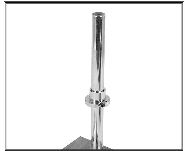
Figure 6. Collar and spacer installed on the column.
