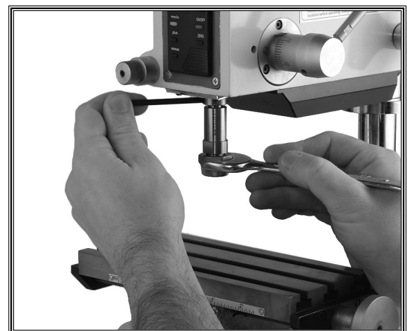
Figure 25. Installing a collet.
