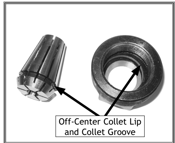
Figure 24. Collet and collet nut lip.
