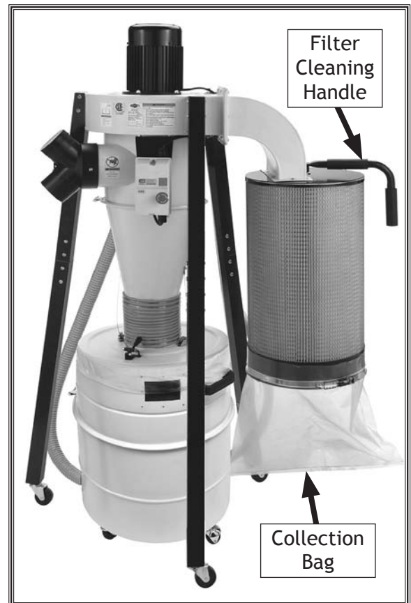
Figure 36. Canister filter and bag.
