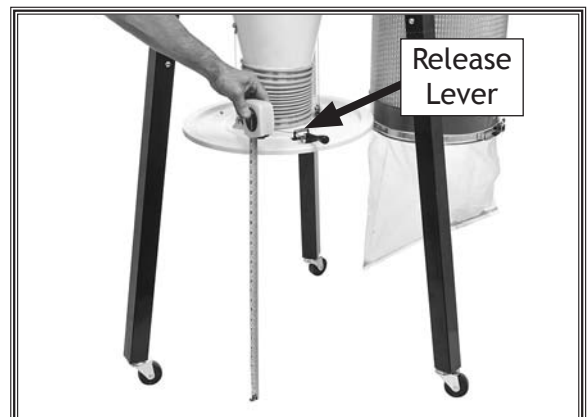
Figure 21. Checking collection lid lift.
