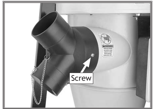
Figure 16. Inlet Y-adapter installed.
