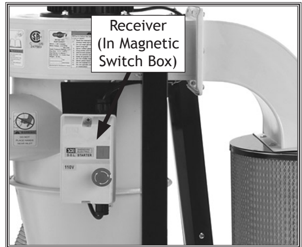
Figure 32. Remote control receiver.
