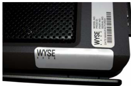
Figure 8 Placement of Wyse Conversion Label
