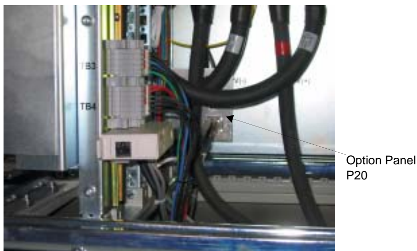
Figure 2-10 GT100E MS Interface Assembly Cable Connection
