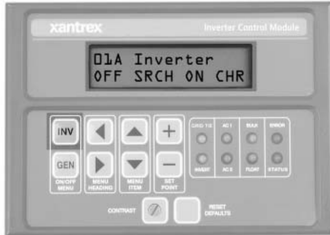
Figure 8-6 Inverter ON/OFF Display
