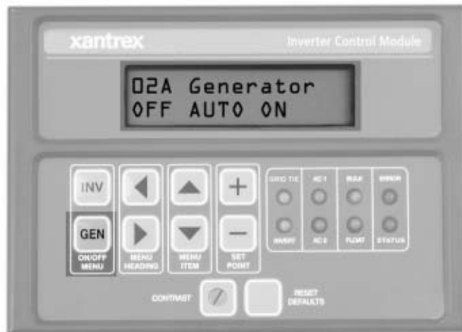
Figure 8-7 Generator ON/OFF Display
