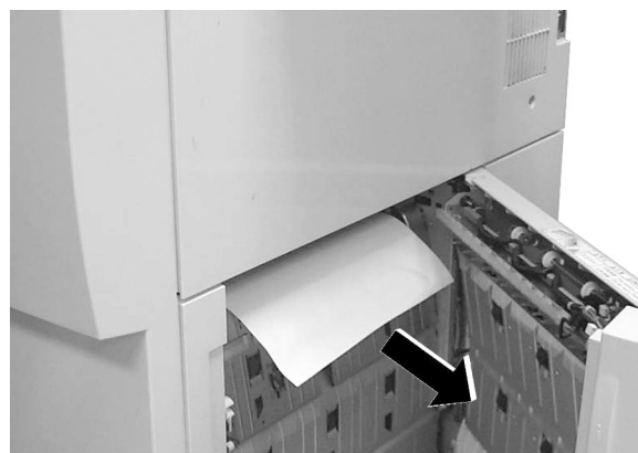
Figure 11: Removing paper behind the copier/printer Right Door
