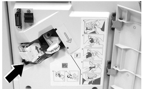
Figure 8: Inserting the Staple Cartridge in the cartridge holder
