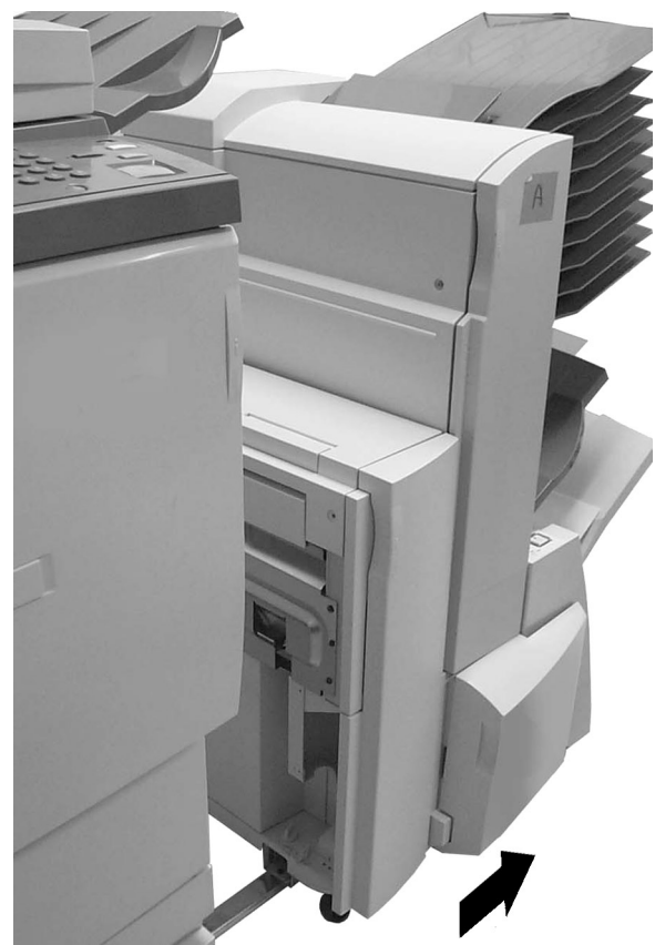
Figure 9: Moving the Finisher away from the copier/printer
