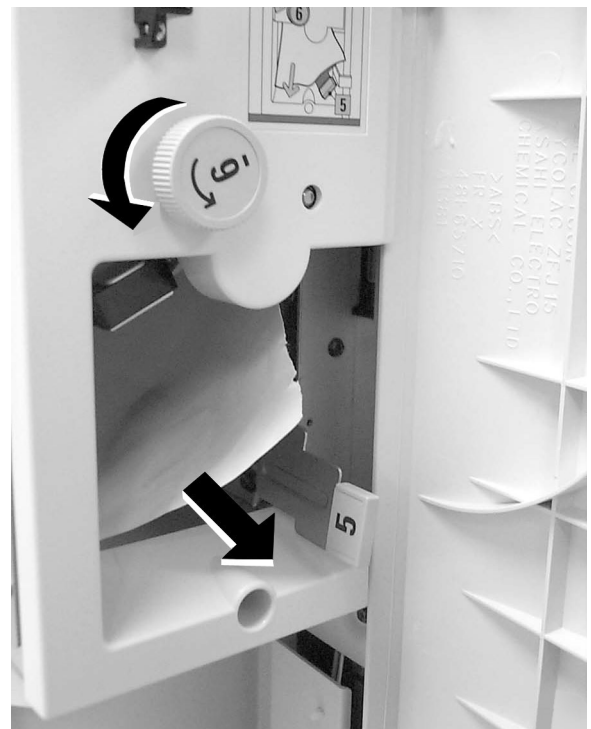
Figure 13: Rotating Knob 6 and removing the jammed paper
