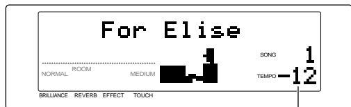
Displays playback tempo as an offset (-99 to +99) from the piano song's internal tempo setting. A TEMPO indication of "---" means that playback is at the song's preset tempo.
