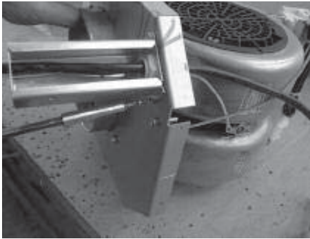
6. Attach junction box to internal flange using provided 1/2" self tapping screws and 4mm internal diameter washers.
