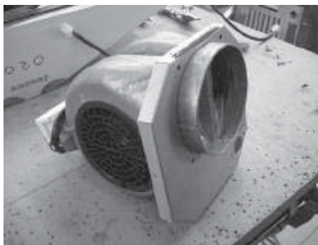
4. Position internal flange over blower housing.
