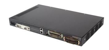
Zhone's 4900 series of ADSL2 + 1U DSLAMs are ADSL ITU G.992.5 compliant IP DSLAMs, Ethernet based, environmentally hardened and small enough to fit in even the most crowded Remote Terminals/Street Cabinets. The 4929 uses EAPS for Ethernet ring topology support, for use with the IPD12000E DSLAM or other EAPS devices.
