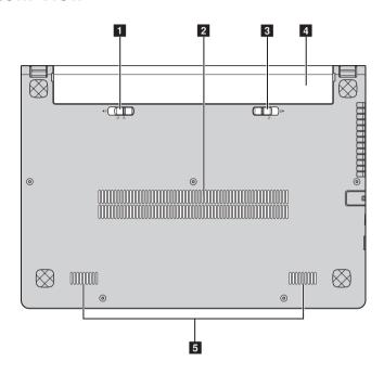
Battery latch - The manual battery latch is used to keep the battery pack secured in place.
