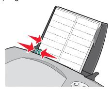
**Note:** If you are using letter size sheets of labels, adjusting the paper guide may not be necessary.
