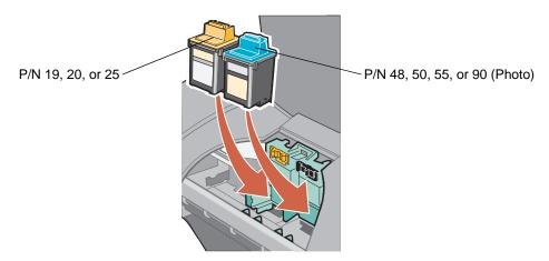
**Note:** To extend the life of your color cartridge and improve printing speed, install a black or photo cartridge along with the color cartridge.
