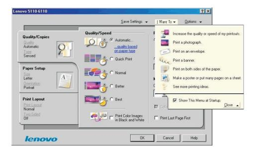
You can change your printer settings in the printer driver. To print a typical document on plain paper, you do not need to change your printer settings. When you install the printer software, the Print Properties are set to these default settings:
