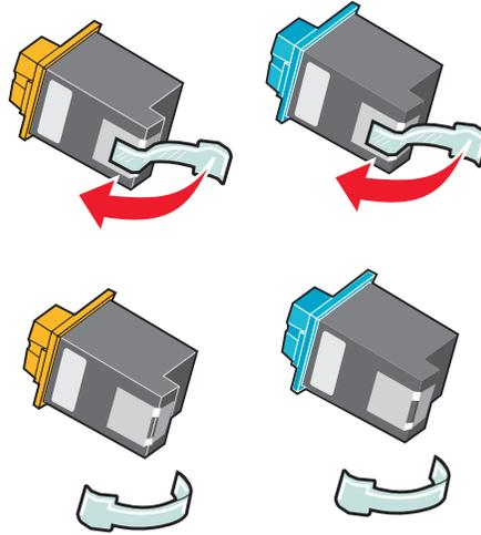
**Warning:** Do *not* touch or remove the gold contact areas on the back and bottom of the cartridges.
