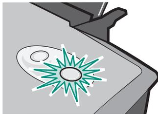
The print cartridge carrier is stalled.
