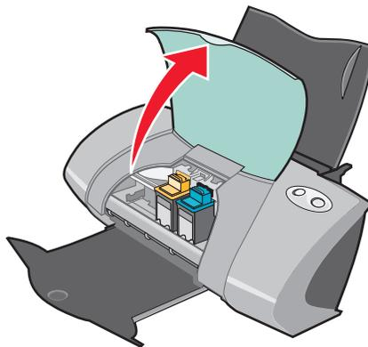
The cartridge carrier moves to the loading position, unless the printer is busy.
