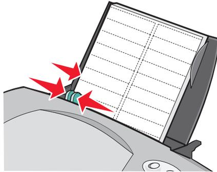
**Note:** If you are using letter size sheets of labels, adjusting the paper guide may not be necessary.
