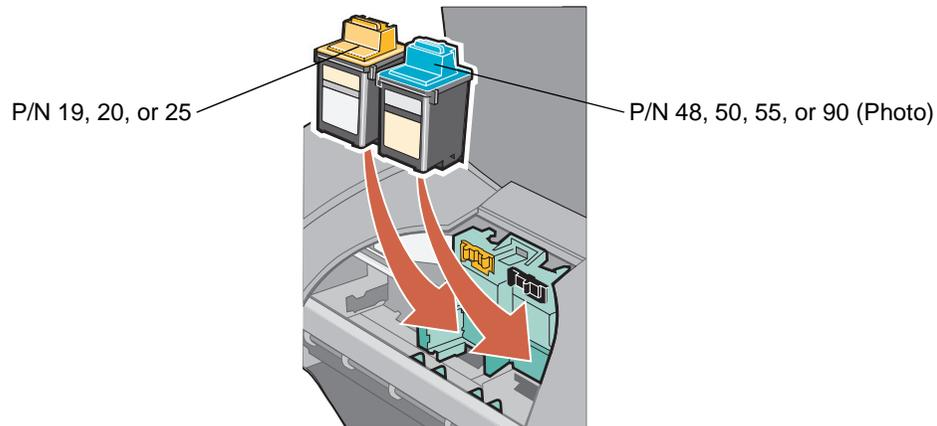
**Note:** To extend the life of your color cartridge and improve printing speed, install a black or photo cartridge along with the color cartridge.
