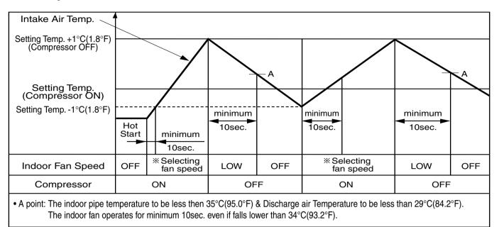
\* During heating operation, the operating procedure of the indoor fan is as the following.
