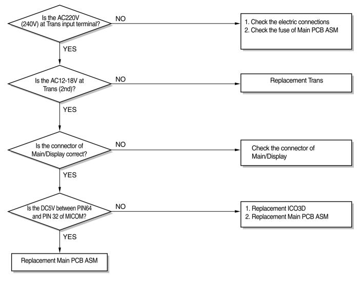
6) Timer control does not operate. Replacement Micom
