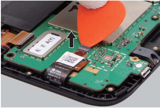
Figure 8. Removal steps of system board (continued) Insert the guitar pick to unsnap the connector.
