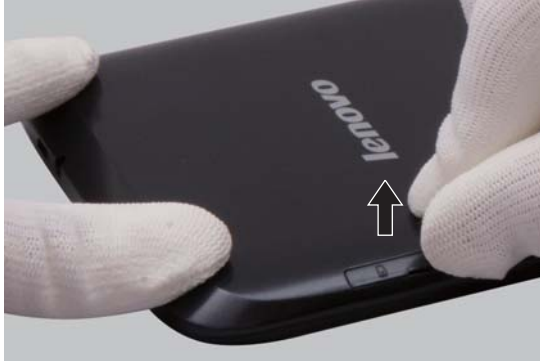
Figure 3. Removal steps of back cover
