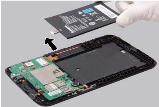
Figure 6. Removal steps of battery pack (continued)
