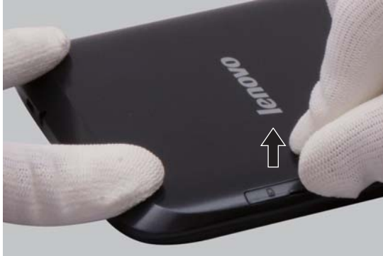
Figure 2. Removal steps of Micro SD card
