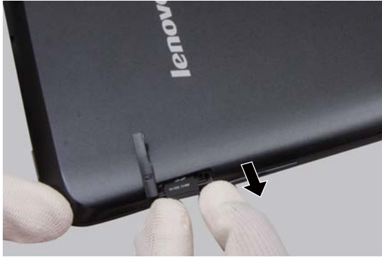
Figure 2. Removal steps of Micro SD card (continued)
