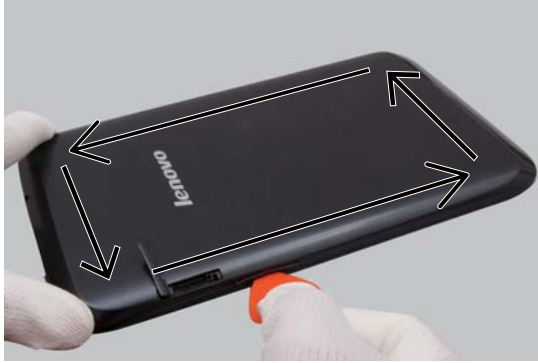
Figure 3. Removal steps of back cover (continued)
