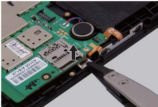
Figure 8. Removal steps of system board
