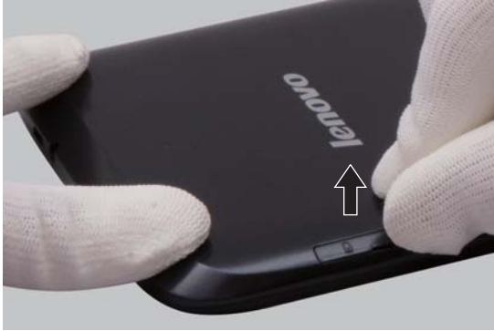
Figure 1. Removal steps of SD card cover
