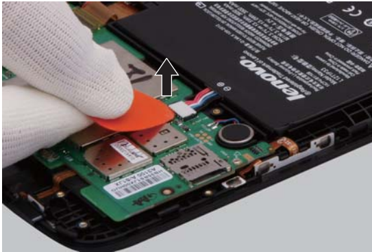
Figure 6. Removal steps of battery pack
