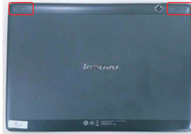
Figure 1. Removal steps of back cover
