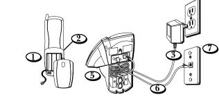
. Remove the battery compartment door on the handset, insert the battery pack, plug the cord into the jack (inside the compartment), and replace the compartment door.
