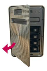
3 Unlock the hard disk rack and pull the lever to draw out the rack.
