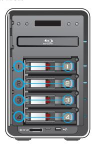
© Keeping the locker lever out, push the hard disk rack into place, listening for the sound. When the hard disk rack is properly and completely pushed in, press the secure button to lock it.
