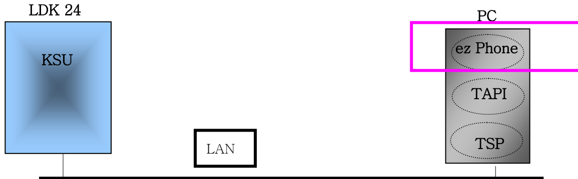
[Figure 1] LDK - 'ez Phone' System Block Diagram (1st Party)
