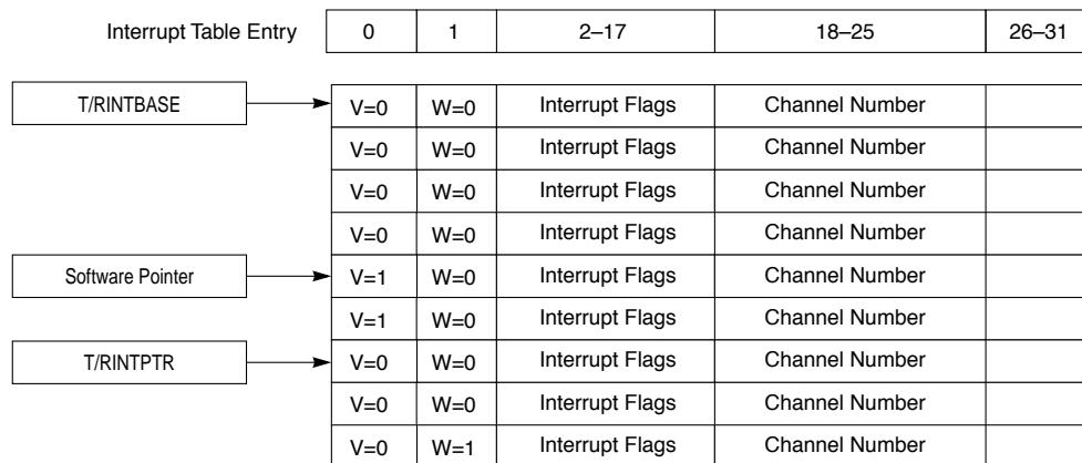
Figure 27-12. Interrupt Circular Table
