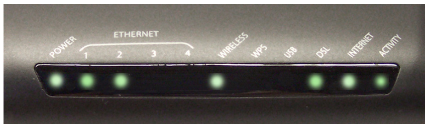
LEDS SHOWING NORMAL OPERATION
