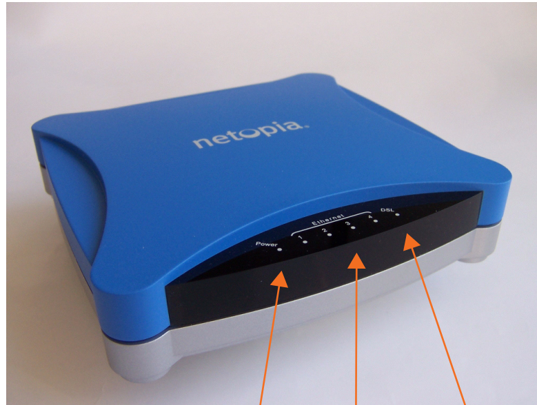
Power Ethernet 1, 2, 3, 4 DSL
